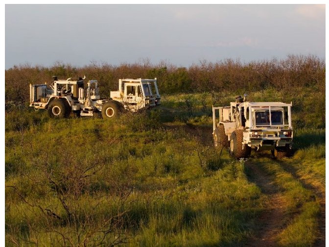
Vibrator Trucks running in Pairs
